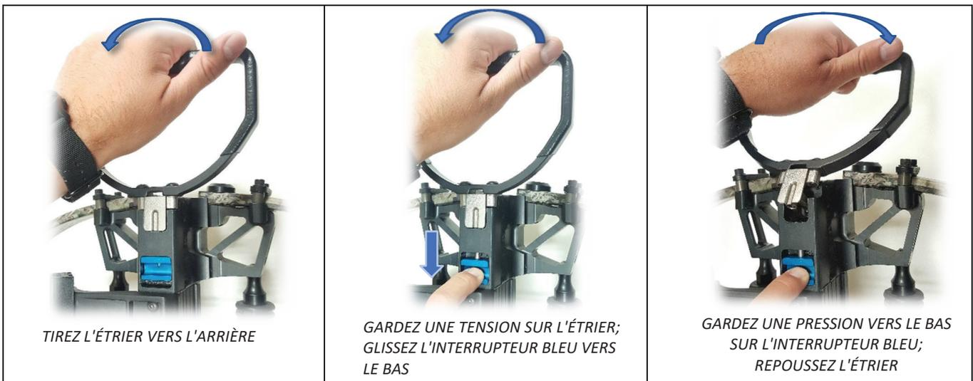
2. TENEZ LE CENTRE PAR LA PIÈCE RACCORD EN PASSANT VOTRE MAIN PAR L'ÉTRIER, PAR-DESSUS L'ESPACE CONSACRÉ À LA POINTE DE CHASSE; TIREZ SUR ASSEMBLAGE DE LA PIÈCE RACCORD EN LA RETIRANT DU CADRE TOUT EN TENANT LES DEUX PARTIES FERMEMENT
