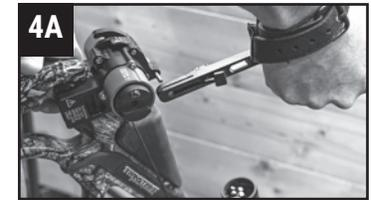
5. Move safety DOWN into the "FIRE" position. The safety must be in the fire position to engage the string catch when cocking. Begin loading the crossbow by turning the handle in a clockwise direction until the string is caught by the string catch. Stop cranking when you hear an audible "CLICK". Visually inspect the string is locked into the trigger catch.
