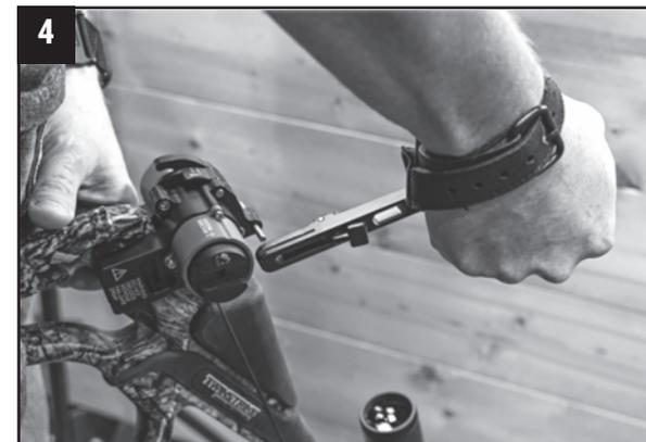
Apply slight pressure to the REAR (lower deck) trigger while rotating the crank handle clockwise with increasing pressure. Once the trigger activates, full draw weight will be transferred to the crank.
