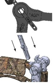
**Step 5**: Move safety up into the "FIRE" position. The safety must be in the fire position to engage the string catch when cocking.
