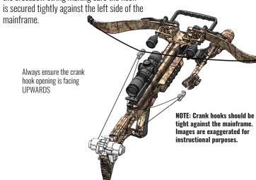
**Step 3**: Run the crank rope around the string groove (located on the stock under the safety) and down the right side of the mainframe and hook onto the string. Confirm both hooks are tight against the mainframe.
