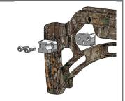
**Step 2**: Slide Charger EXT into bracket on the and push down. You will hear an audible "CLICK" when properly engaged. Verify by pulling up on the crank.
