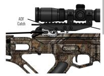
**Step 6**: Once you have confirmed that the trigger catch has captured the crossbow string. Immediately place the safety into the "SAFE" by moving it into the down position.
