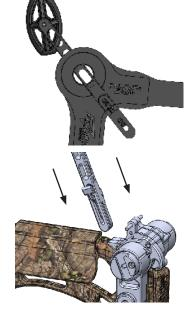
**Step 2**: Keeping a firm grip on the crank handle, move safety up into the "FIRE" position.
