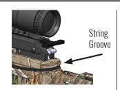
NOTE: IF THE HOOKS ARE JUMPING ON TOP OF THE MAINFRAME WHILE CRANKING YOU HAVE NOT BRACED THE ROPE THROUGH THE STRING GROOVE LOCATED UNDER THE SAFETY (SEE IMAGE). THE HOOKS CAN DAMAGE THE SIDE OF THE MAINFRAME IF THE ROPE IS NOT POSITIONED CORRECTLY. DAMAGE CAUSED BY INCORRECT USE OF THIS COCKING AID IS NOT COVERED UNDER WARRANTY!
